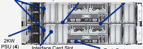
Interface Card Slot (6x2 adapter cards) (up to 24 ports per 2U)
